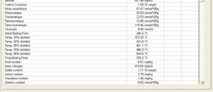
Figure 4. Toplab FCC feed characterisation screen display.
